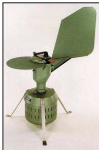
Fig. 1: A Burkard 7-day recording volumetric spore trap
